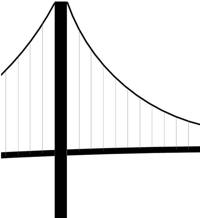
**Cable Suspension** By using cable wires in suspension (i.e., in tension vs. in compression), the cables could be very thin and elegant as there is no threat of buckling in tension. This thinness gives the structure an elegant expression. The viewer does not see a support system struggling to bear 61,500 tons—as with arched/compression bridges—but rather is impressed with the overall expression of lightness and grace.
