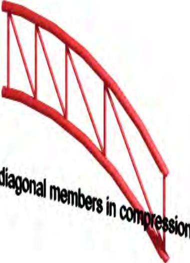
**Arches** The arches supporting the portion of the bridge on the land have inward sloping diagonal members, which puts them in tension, the optimum condition given that they are composed of steel. Although the nature of the arch makes for all elements to be in compression, placing the diagonal members in this way puts them in tension, and thus allows for the members to be thinner without threat of buckling.
