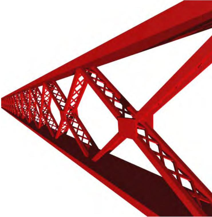
**Trusses within Trusses** The steel trusses exploit steel's tensile capacity and maximize its efficiency by removing bulk which does little or no work. If this were not the case, much of the steel's structural capacity would be wasted supporting itself, resulting in an extremely inefficient system. In addition, the increased mass would increase the seismic force on the structure.
