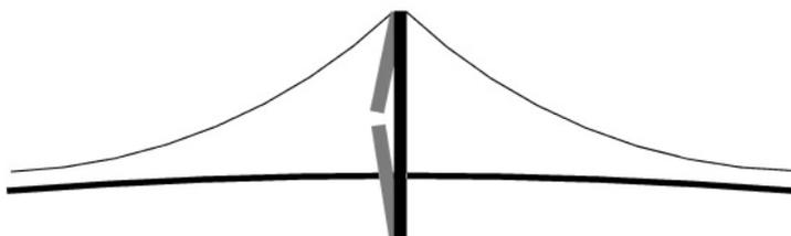
**Funicular Structures** Many steel bridges use arches as the key structural component, and resemble an upside-down Golden Gate bridge. Such a structure would have been much less efficient for several reasons, including:
