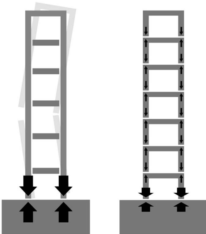
**Stacked Towers** The towers are composed of separate upside-down U-shaped members stacked on top of one another, as opposed to being made of two tall posts which stretch the entire height and horizontal connections. This better distributes the forces on the towers (106,000 tons) and reduces chances of buckling. It also reduces the chances of cracking/failure in unexpected places by essentially predefining (and reinforcing) the vulnerable points.
