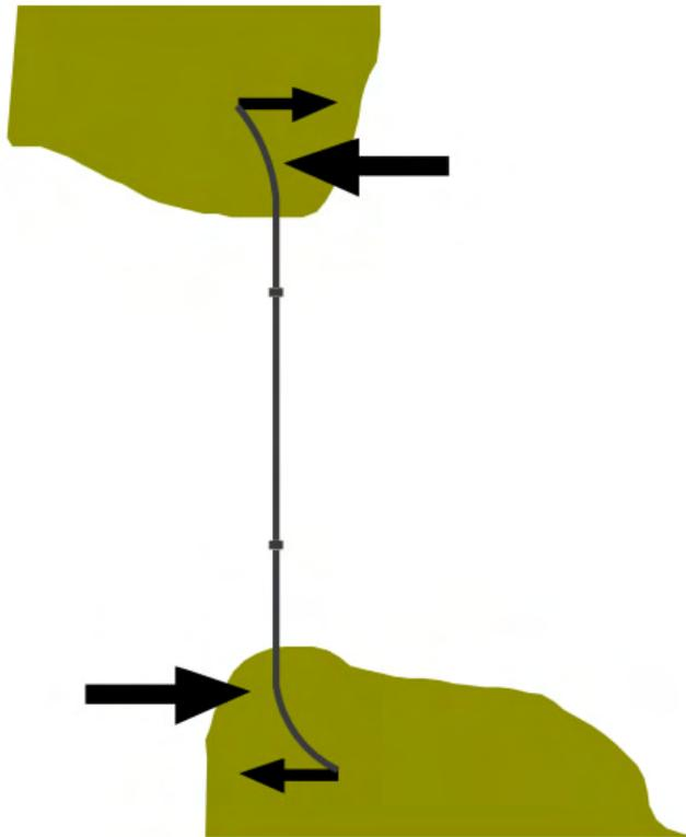
**Curved Ends** The approaches to the bridge are curved at each end to increase lateral resistance and thereby prevent the entire structure from overturning or rotating along its axis.
