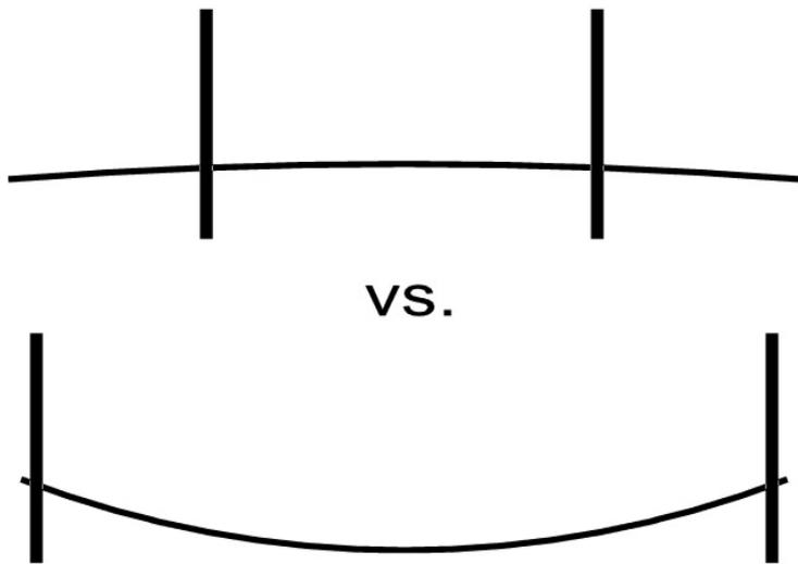
**Cantilever** The upward curve of the bridge greatly reduces positive bending, which is essential for such a long span of 6450 feet. This is enhanced by strategic placement of the towers. Rather than being on each end, the towers are located away from the edges so that the bridge cantilevers on either end, causing negative bending which counteracts the positive bending. This significantly reduces the amount of steel necessary in the bridge.
