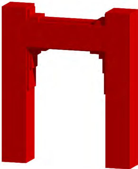
**Moment Frames** The towers have moment frames to resist shear and overturning. While braces could have done the job similarly, the moment frames allow for openness and a less structure-dominant, more aesthetic look. The fact that X-braces are used on the towers only under the bridge (hidden from common view) further this idea of synergy of structure.
