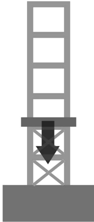
**X-Brace** The tower has X-braced moment frames beneath the bridge to provide additional lateral resistance and compressive strength (due to the added weight of the bridge itself).
